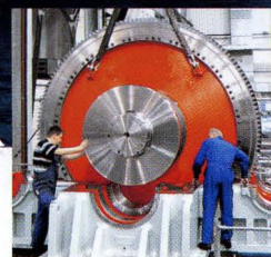
Double marine gears from Rheine plant for the LNG tanker called "Gaz de France"
